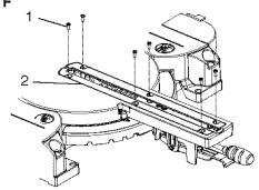
MOUNTING THE MITER SAW (FIG. G, G-1)
